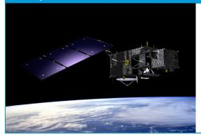
Sentinel-3 is an ocean and land mission composed of three versatile satellites(Sentinel-3A, Sentinel-3B and Sentinel-3C). Sentinel-3A's ocean and land colour instrument can 'see' chlorophyll in vegetation. The amount of chlorophyll present in plants plays an important role in determining how healthy they are. Monitoring chlorophyll from space provides a valuable tool to support vegetation management, agriculture and forestry.
